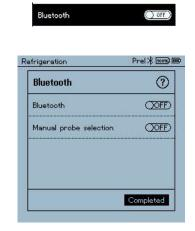
When the Bluetooth<sup>®</sup> icon is not shown on the display, Bluetooth<sup>®</sup> is switched off.
