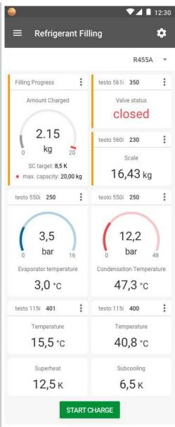
Added refrigerant is displayed in g/kg increments on the manifold/app.
