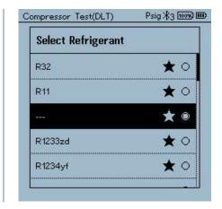
Setting the refrigerant: Press [▲] or [▼] to select the refrigerant and press [Menu/Enter] to confirm.
