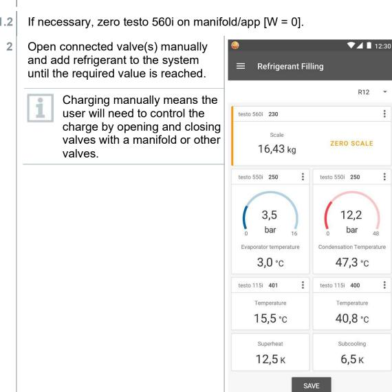
Added refrigerant is displayed in g/kg increments on the manifold/app.
