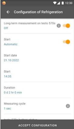
If the long-term measurement option is enabled, the configuration menu shows the remaining battery and rechargeable battery capacity and the maximum possible duration of the long-term measurement.
