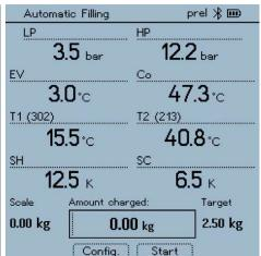
4 Once charging is finished, the process can be repeated [NEW] or another mode for charging [OPTIMIZE] can be selected.
