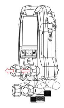
2 Fold out the suspension device, release the clip, remove the battery compartment cover and remove the batteries.
