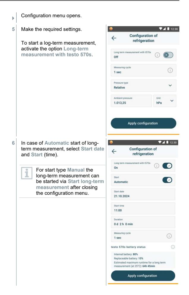
If the long-term measurement option is enabled, the configuration menu shows the remaining battery and rechargeable battery capacity and the maximum possible duration of the long-term measurement.
