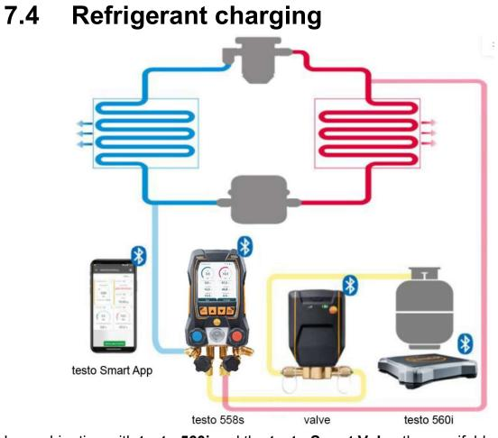
In combination with **testo 560i** and the **testo Smart Valve** the manifold **testo 558s** offers multiple functions to charge refrigerant systems.
