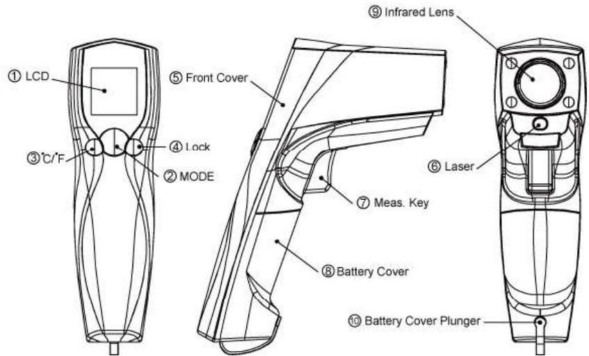
Simply aim the thermometer at the measure target with Lens (9) and press Meas. key (7) to display the surface temperature. The Distance:Spot is 12:1. Please make sure the target area is within the field of view.
