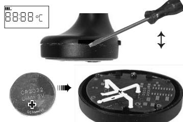
The battery has to be changed if appears in the display during the measurement. Open the housing using a screwdriver. Remove the used button cell. Put in new button cell - Observe polarisation!
