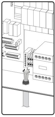
**C.-** Put on the cover, and arrange the wiring according to the diagrams enclosed. Connect the control hose (1), adjust the motor guard (Q1/Q3) and close the cover (2).
